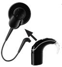
1. Hold the coil cable grip and firmly pull it straight out of the processor. Do not pull on the flexible part of the coil cable.
