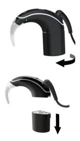
Twist the battery module as shown to release it from the processing unit.
