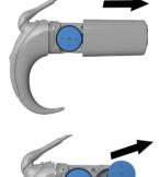
3. Remove the batteries from the battery holder.
