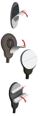
Peel off the single backing strip on the adhesive side of the pad.
